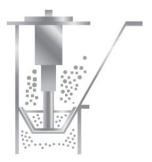
Unprocessed material is **UnaidMill** into the product **invertion** gravity feed or vacuum transfer. The material is instantly reduced in size as it passes through the holes in the screen.
