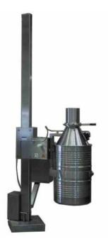
The **Uni-Hoist** range now has two separate designs. A lightweight version for loads up to approximately 600kgs and a heavy duty version for loads up to 1250kgs. Smaller hoists can be manually operated to provide a cost effective solution for light loads.
