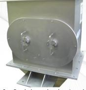
The SureBreak lump breaker is a low speed machine that reduces the product by a cutting and sheering action. Furthermore, no grinding takes place during the size reduction process, resulting in no heat generation, less noise and no metal-to-metal contact.
